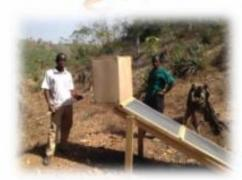
A food drier requires air movement and heat to generate necessary air flow to dry fruits and vegetables.
